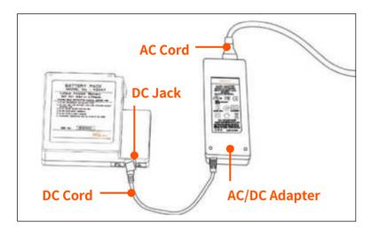
Make sure the voltage and frequency and connect the DC cord of the AC/DC adapter to the DC jack of the battery. The LED turns to green when the charging is completed. The battery includes the protection circuit that prevents full discharge and full charge. The supply of power stops once the protection circuit is activated. In order to deactivate the protection circuit and resume feeding power, wait about 10 seconds and connect again the DC cord to the DC jack.
