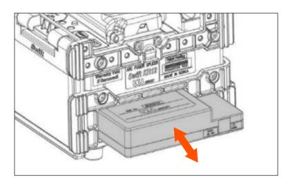
**Inserting the Battery**
