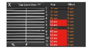
It is displayed when the measured gap of the fiber is greater than the limit.
