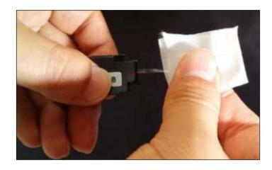
Clean carefully the fiber with a piece of soft cloth or gauze soaked in alcohol.
