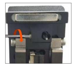
Mode change Adjust gear pusher position after loosen Set-screw as shown picture.
