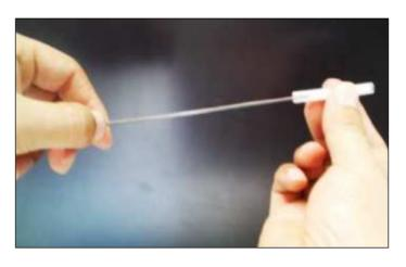
Insert the fiber into the sleeve.
