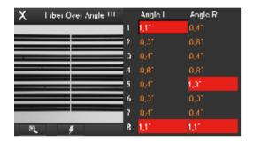
It is displayed when the measured cleaving angle of the fiber is greater than the limit.
