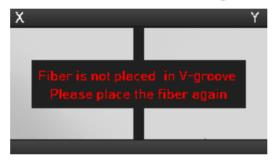
It is displayed when the fiber is not placed on the V-Groove.
