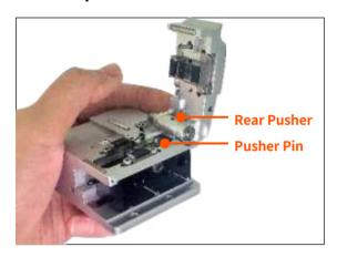
1 In order to replace blade, disassemble chip collector assembly and rear pusher. Open the cover as shown picture and press the pusher pin to move slider to forward.
