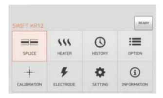
To import splice mode, press and select icon by touch. It displays a screen to select splice mode as above. The selecting screen is equipped with various splice modes to facilitate a user's easy selection and use of splice mode. In addition, splice mode can be expanded and saved up to 300 units. These splice modes are classified into general mode and user mode.
