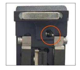
**Blade locking mode.** When the blade is used without rotating.
