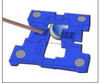
Any contaminants inside the V-groove will affect the splicing condition of the fiber, resulting in higher splice loss. Hence, it is important to inspect the V-groove often and clean it periodically in accordance with following ways.
