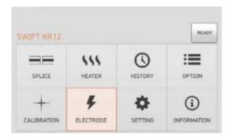
In normal operation mode, to call the Electrode menu, press MENU Then you can see the Electrode menu as above. It is necessary to regularly check and clean the electrodes because they are worn out. The silica oxidized substances is deposited as the electrodes go through numerous times of splices. There're already various functions to arc count, replace time and other.
