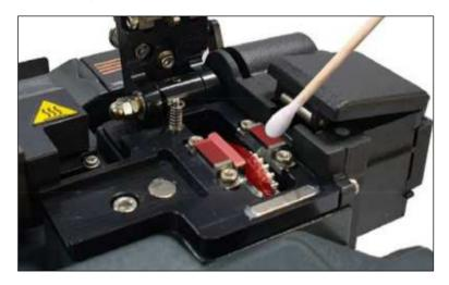
The performance of the fiber cleaver can be deteriorated if the blade or clamp pads of the cleaver are contaminated. In addition, the contamination of the fiber surface or tip can cause higher splice loss. For this reason, it is important to clean both the blade and clamp pads of the cleaver with a cotton swab soaked in alcohol.
