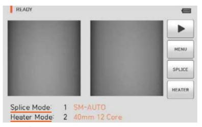
Press and hold for about 1.0 second without opening the windshield cover. The initial screen is displayed as above after resetting all their initial functions. It is important to choose a right splice and heat mode to ensure an accurate splicing result. The current splice, heater and stripper mode are displayed at the bottom of the initial page.
