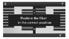
It is displayed when the fiber is not placed in the middle of the electrodes and V⊠groove or the objective lenses or reflection mirror is contaminated.
