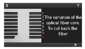
It is displayed when the measured variation of the fiber length is greater than the limit.
