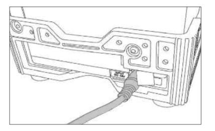
Swift KR12 can be charged during operation because the floating charging method is applied. The battery can be also charged with 12V Cigar jack charger.
