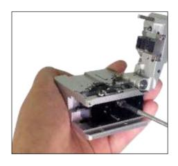
**2** Remove blade pin completely using (-) driver.
