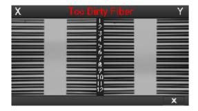
It is displayed when the fiber prepared for splice is contaminated more than normal status.
