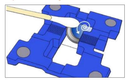
The contamination of the objective lenses surface may cause inaccurate observation of the fiber position, resulting in higher splice loss and poor performance of the Swift KR12. Therefore, the two objective lenses have to be cleaned on a regular basis. Otherwise, the dust sticks on the surface and it may become irremovable eventually.
