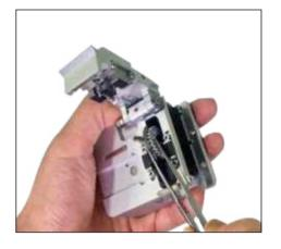
3 Remove old blade with blade gear from body and replace new blade with blade gear. In here reassembling should be done in a reverse order of disassembling. At this time, especially be careful not to damage the blade. Check the blade operating condition with cleaver cover.
