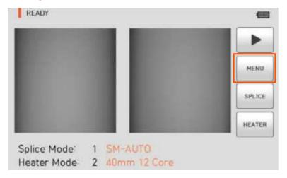
Main menu has 8 submenus. Press MENU or touch the MENU icon on the screen to load main menu. The main menu screen is as above. You can select right and left by pressing HEAT and SET buttons.
