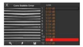
It is displayed when bubbles or dots exist in the spliced part after completing the splice.
