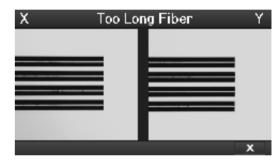
It is displayed when the fiber is placed too close to the electrode, the lenses or reflection mirror is dirty or LED light is not bright enough.
